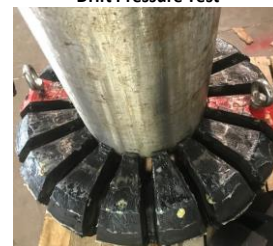
Annular BOP – Packing Element Drift Pressure Test
