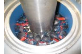
Ram BOP – Front Packers, Top Seals & Door Seal Function Pressure Test
