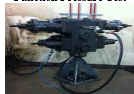
Ram BOP – Front Packers, Top Seals & Door Seal Function Pressure Test
