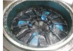
Annular BOP – Packing Element Drift Pressure Test
