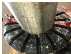
Annular BOP – Packing Element Drift Pressure Test
