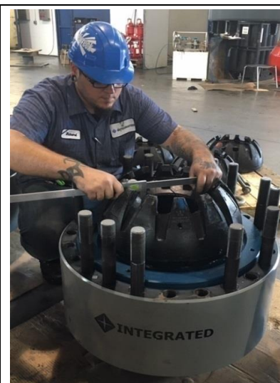
ANNULAR INSPECTION PRIOR TO SEAL & PACKING ELEMENT INSTALLATION
